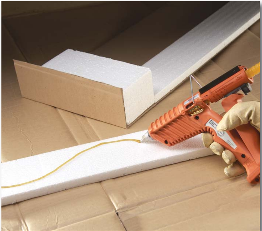
3M™ Scotch-Weld™ Hot Melt Applicator LT with 3M low temperature (265°F/129°C) adhesive effectively bonds heat-sensitive substrates such as styrene foam to itself, corrugated, or other surfaces without damaging the foam.
