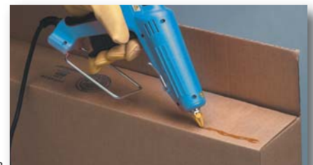
Self-contained portable 3M applicators save the cost of bulk equipment for recoupage, manual random size case sealing, and many contract packaging situations.
