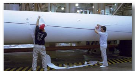
318 For finished mill overlap splicing, 3M™ Repulpable Permanent Tape provides high shear strength without adhesive oozing or bleed through.
