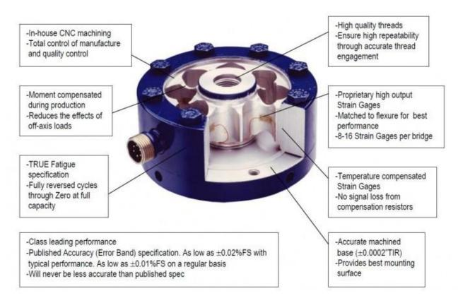
Every Interface low profile load cell is moment compensated during production, the proprietary strain gauges offer outputs as high as 4.0 mV/V, fatigue rated units are warranted for 100 million fully reversed cycles from full-scale Tension through Zero to full-scale Compression.
