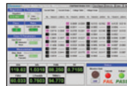
IEC 61000-3-2 Current Harmonic Test (Pre-compliance)
