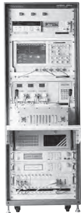
DC to DC Converter ATS
